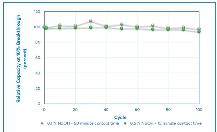
Each cycle represents equilibration, load, wash, elute and CIP with 3CV NaOH. Alkaline stability evaluation was performed at 4° C.
